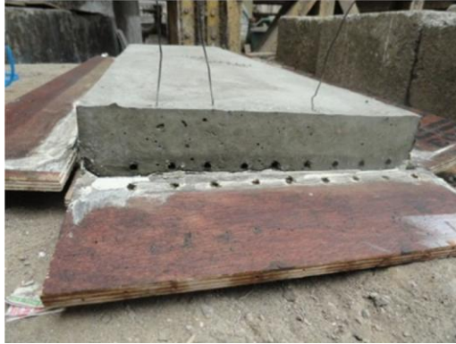
Slab specimen after removal of shutter with hollow duct to fill with resin Fig. 3
