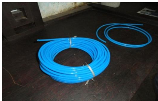
Void Former (Polyurethane Material) Fig. 1
