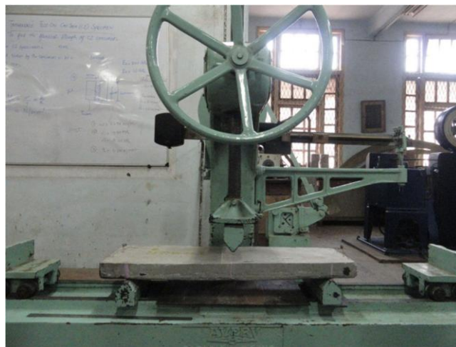
Slab specimen under one point flexural loading system (Ducts filled with resins) Fig. 4
